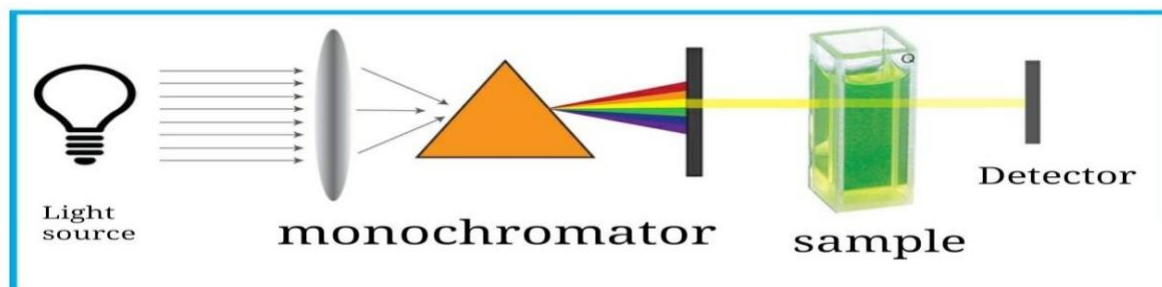
Fig. 2: Instrumentation of UV-Visible spectrophotometer
